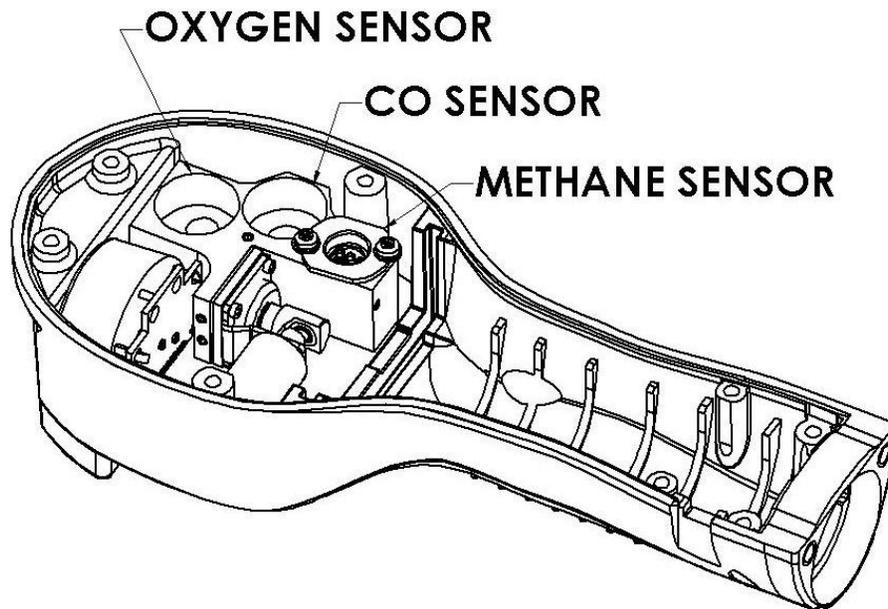
**Figure 4.** Gas-Explorer with top of case and main circuit board removed.
